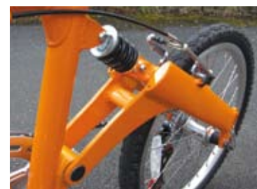
Components on the Downtube are generally of good quality. They say the stem has been improved to eliminate the play present on our sample. Having bar ends fitted as standard is a pleasant surprise.
