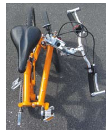
ABOVE: Without a strap to hold the folded package together, the stem tends to swing out sideways.
